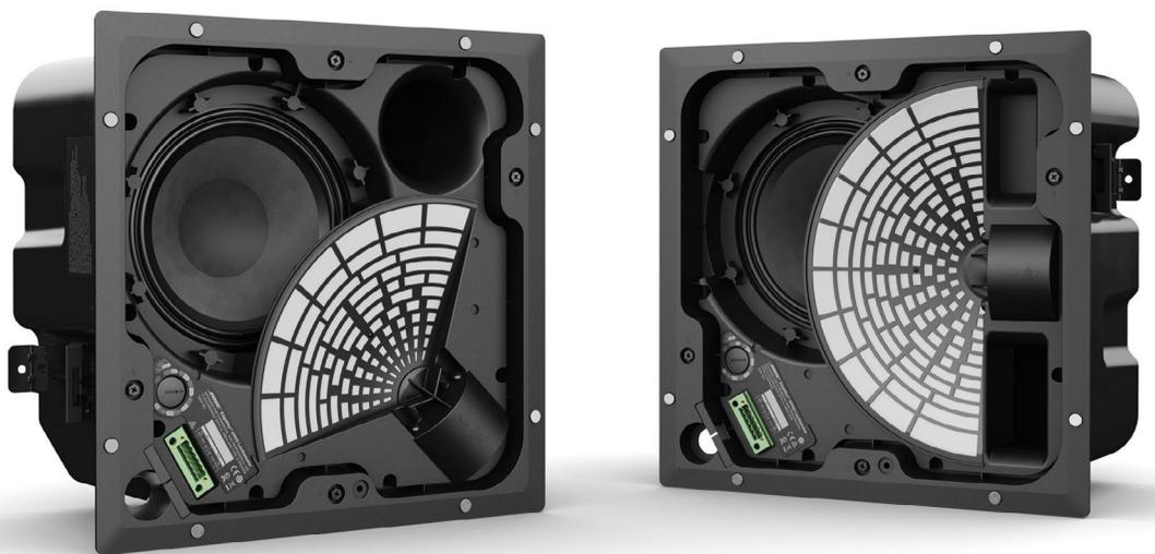
Bose Professional's EdgeMax in-ceiling loudspeakers feature an 8-inch woofer and a 1.4-inch compression driver, incorporate proprietary Bose PhaseGuide technology offering nominal 90- (left) or 180-degree (right) horizontal coverage, and are designed for mounting near wall boundaries.
